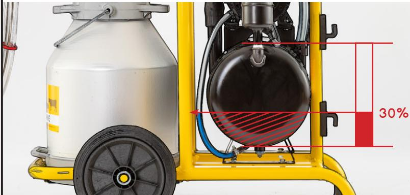
The oil level can be monitored through the transparent thin hose that connects the oil tank to the pump.
