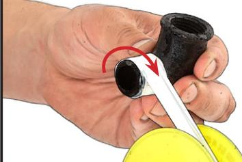
Seal the thread of the exhaust filter with Teflon tape or hemp.
