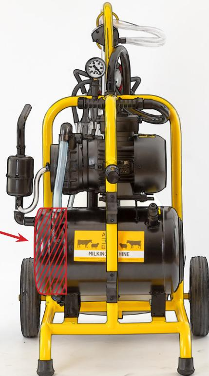
The optimal oil level is about 30% of the tank's total height.
