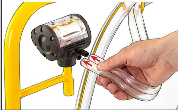
Connect the thick hose(s) on the vacuum manifold to the pulsator bracket(s).
