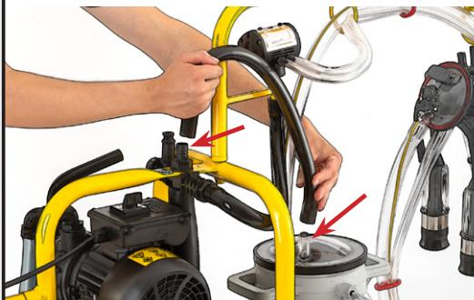
Carefully place the vacuum gauge into its designated position on the machine.
