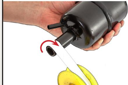
Screw the exhaust filter into the elbow on the vacuum oil tank. Position the exhaust outlet so that it does not interfere with the operator or the animals during milking.
