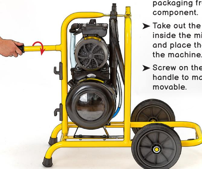
It is recommended to perform the assembly at a temperature above 20 °C to make it easier to fit the hoses. If the hoses are difficult to attach, moisten their interiors with water or gently warm the ends with a heat gun.
